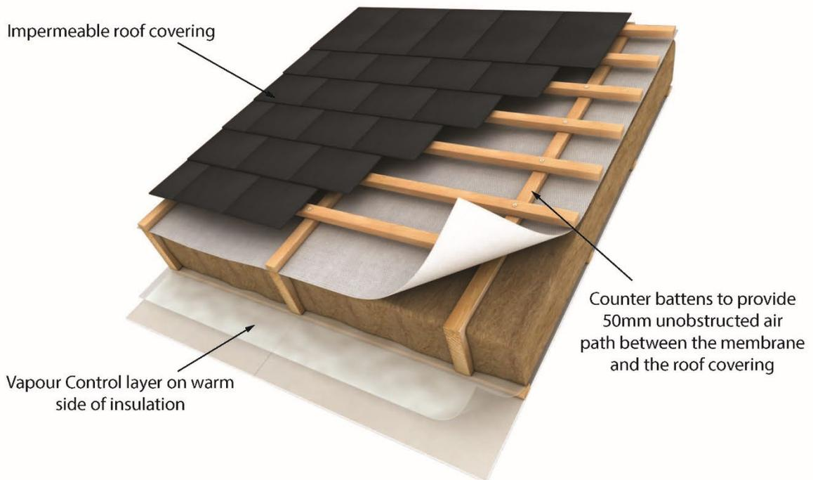
Figure 2: Warm Roof detail with impermeable roof covering
