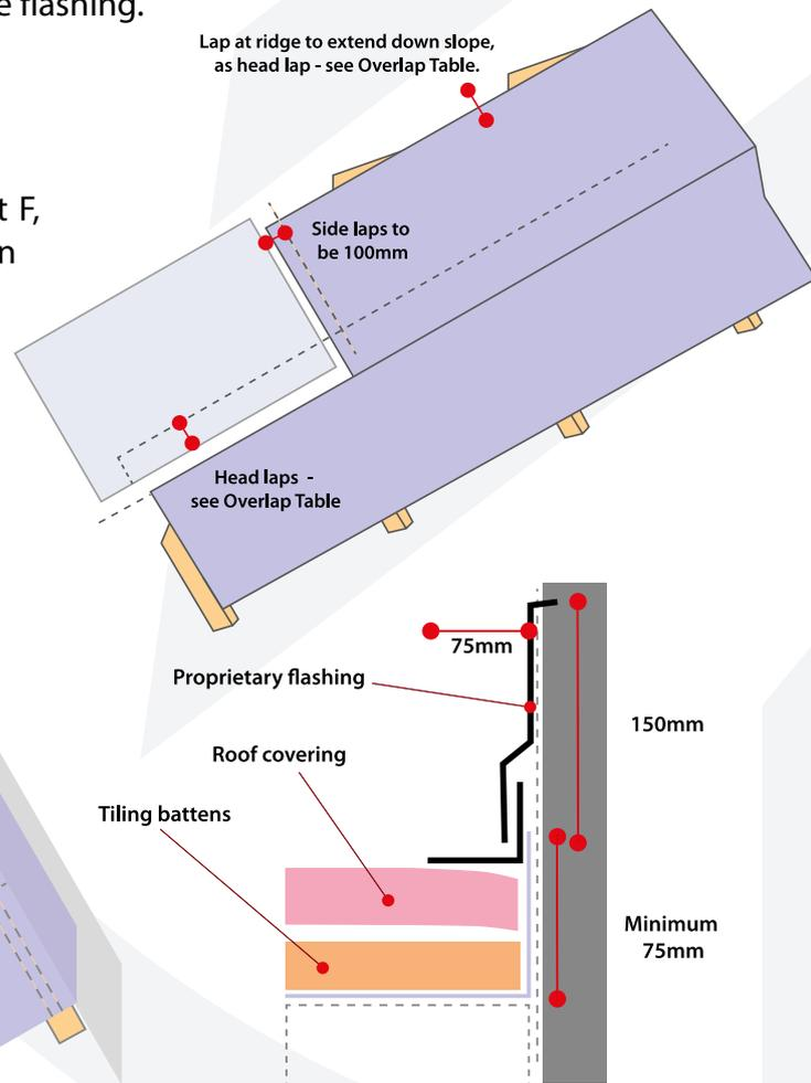
Figure 4 - Abutment Detail
