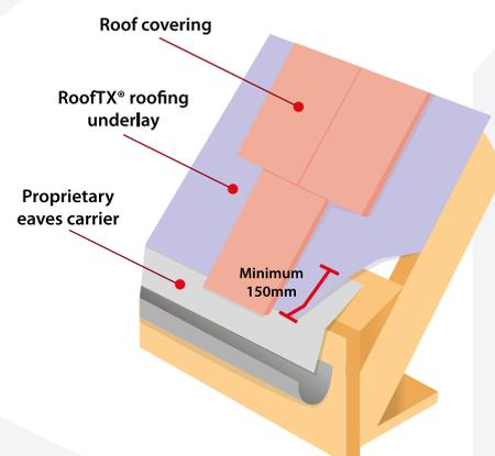
Underlay to extend a minimum of 150mm over proprietary eaves carrier, which must extend beyond the fascia to ensure effective drainage into the gutter
