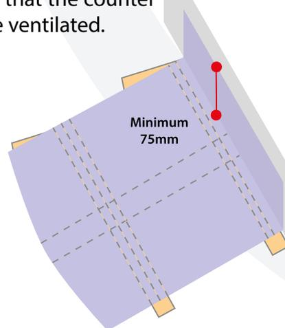
RoofTX® Roofing Underlay to form up-stand of at least 75mm below 150mm deep proprietary flashing
