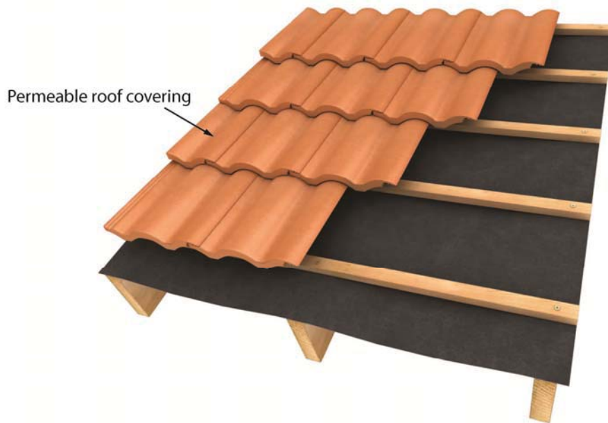
Figure 1: Cold Roof detail with permeable roof covering
